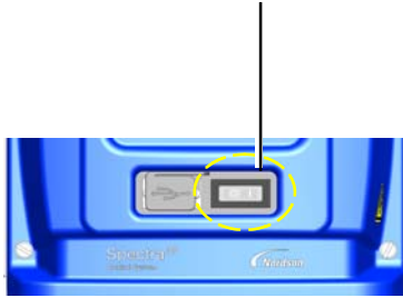
Figure 3-10 Main Switch location
